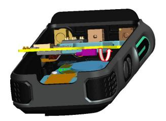
13. Use the slotted screwdriver to open the buckles at the arrows to push out the PTT button (A), rubber (B), holder (C), side key (D and E), holder (F). The holder (C) and the rubber (D/E) can be separated directly.
