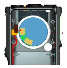
15. To dismantle the MIC, remove the white sealing (A) around the MIC, and use the screwdriver to take it out.
