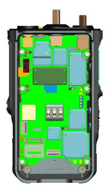
12. Lift the main PCB up obliquely to remove the LCD FPC (A), and take out the main PCB.
