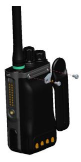
3. Remove the screw of accessory interface cover with slotted screwdriver to remove the accessory interface cover;
