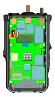
11. Remove the six screws of main PCB with the cross screwdriver;
