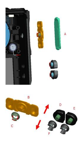
14. To dismantle the speaker, remove the white sealing (A) around the speaker, and use the screwdriver to take it out.
