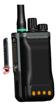
4. Push the battery lock to remove the battery;
