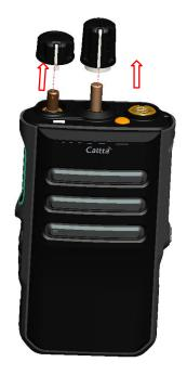
7. Use the sockets to remove the antenna nut and switch nuts;
