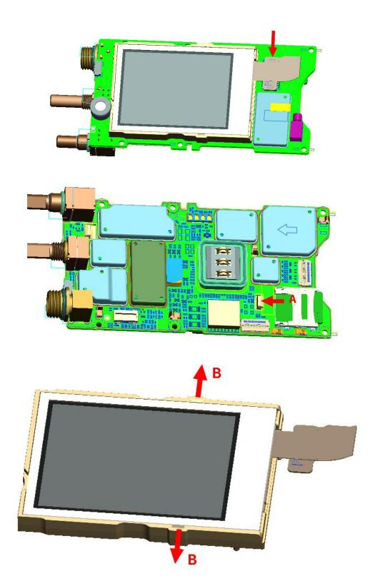
9. Remove the four screws at the arrows with the cross screwdriver to take out the P+R keypad.
