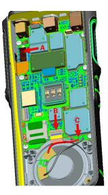
7. Remove the six screws of main PCB with the cross screwdriver to take out the main PCB obliquely, be careful that the accessory interface board FPC and connector can obstruct the main PCB, pay attention to pull it out slowly not to break the FPC with too much force.
