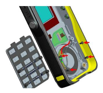
10. Remove the white sealing on the back of keypad at the arrow with the slotted screwdriver after taking out the P+R keypad, press the keypad from the back to remove it.
