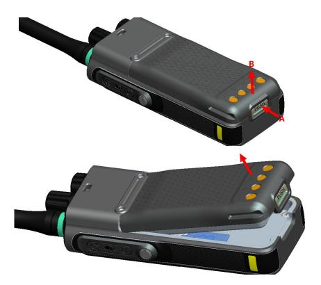
3. Use the T8 screwdriver to remove the two screws at the arrow to remove the aluminum cover component.
