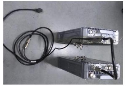
Figure 2-5 Connection between MPU and RRU with the the power line
