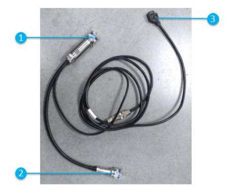
1) A Connector : Waterproof connector with large size diameter, connect to RRU
